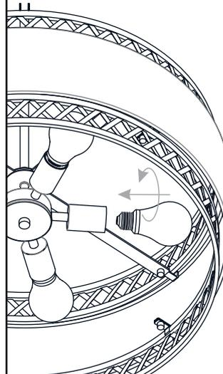
Install five correct bulbs referring to fixture markings and/or labels for maximum wattage.
